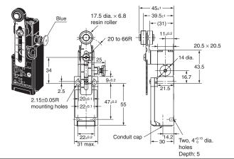
Adjustable Roller Lever, Form Lock (with Metal Lever, Rubber Roller) D4N-1□2HR D4N-2□2HR
