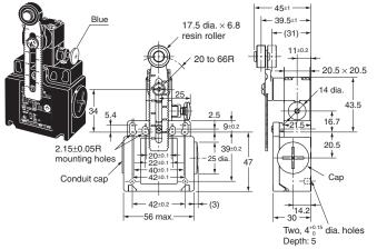
Adjustable Roller Lever, Form Lock (with Metal Lever, Rubber Roller) D4N-6□2HR
