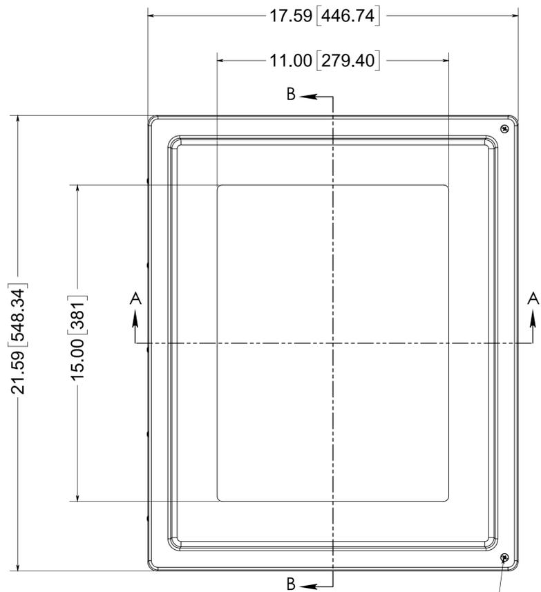
(2X) EACH #10-32 BRASS INSERTS AND 316 STAINLESS STEEL CAPTIVE COVER SCREWS WITH RETAINING O-RING
