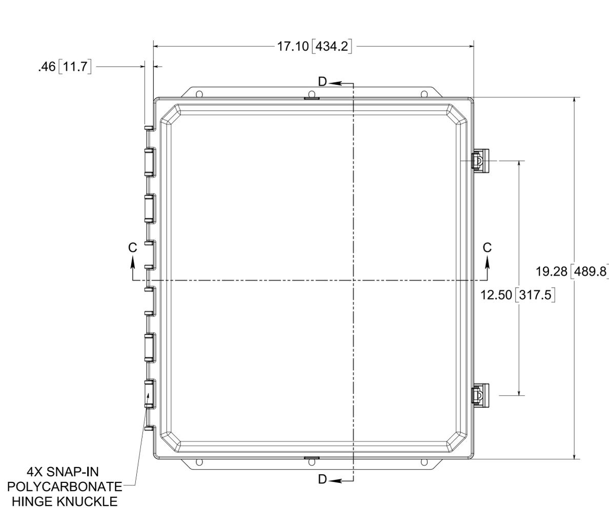
4X SNAP-IN POLYCARBONATE HINGE KNUCKLE
