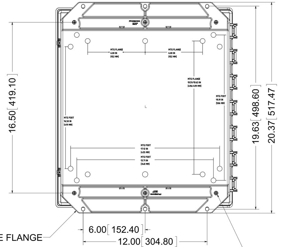
(6) EACH #10-32 BRASS INSERTS AND STAINLESS STEEL FLANGE AND FEET SCREWS
