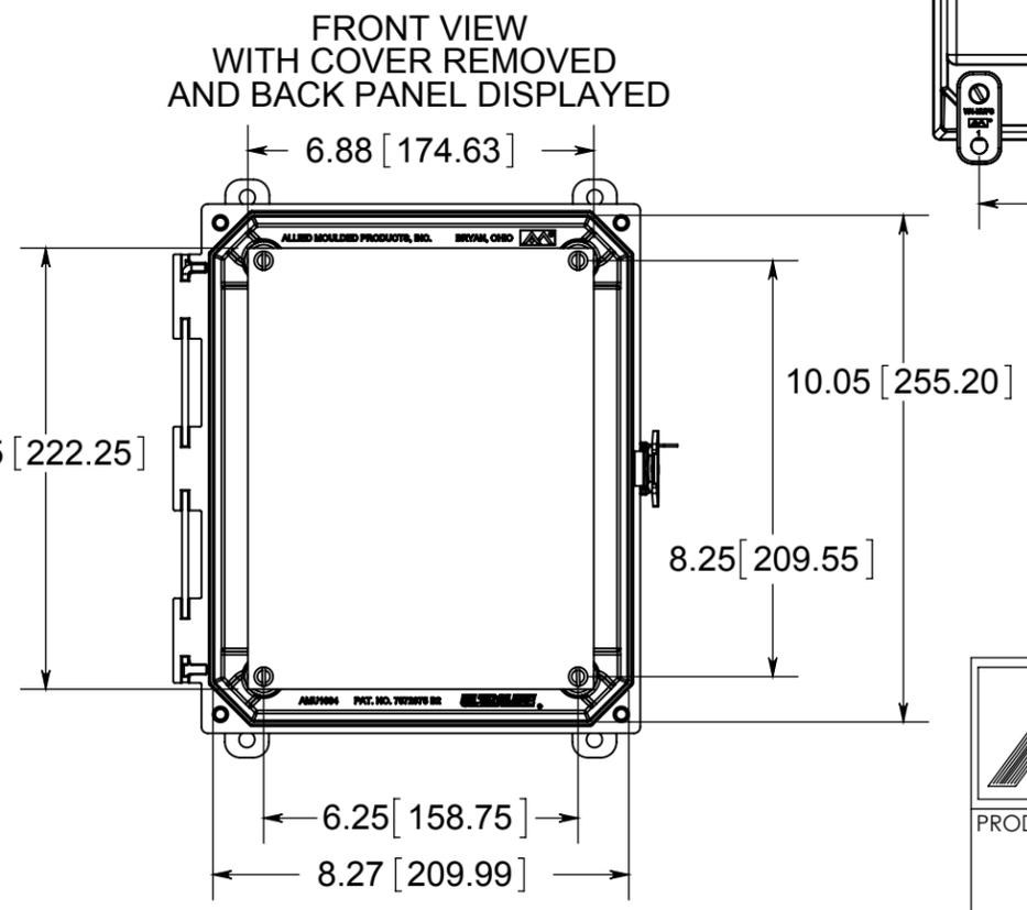
(4) EACH #10-32 BRASS INSERTS AND PLATED CARBON STEEL SCREWS
