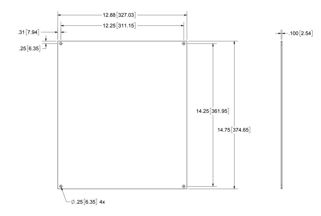
Aluminum 3003-H14 With Protective Peel-Off Film
